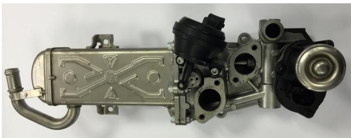
All components are reassembled before the unit is **calibrated** and **tested**. This procedure accurately calibrates the electronic feedback of the valve. The coolant section is then pressure tested to detect any leaks. The final test is to flow gasses through the unit at various pressures and rates to ensure the correct electronic signal is output from the valve
